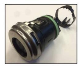
Left: Capless unit with nozzle guide detached for clarity
