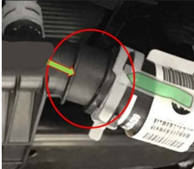
Fig. 1 Lower Radiator Hose Not Fully Seated Against Plastic Stop
