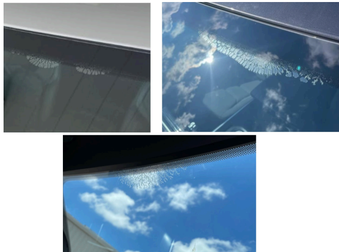
Fig. 1 Examples Of Snowflaking/Delamination
