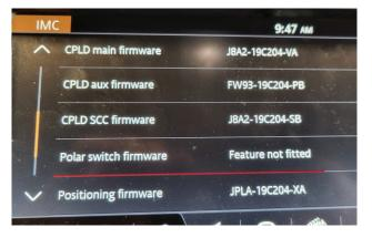
If Polar Switch Firmware does not report and shows "Feature not fitted" recommendation is IMC replacement
