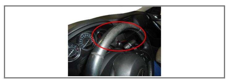
**NOTE:** Slight wear on a seam of the steering wheel is considered normal wear since friction and force are applied while turning the steering wheel.
