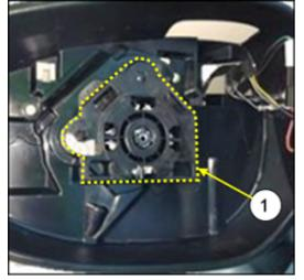
b. Peel off the release papers on the new mirror glass holder.
