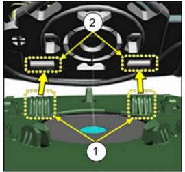
d. Hook the claws (1) of the the outer mirror holder to the pivot plate (2) shown in the following image.
