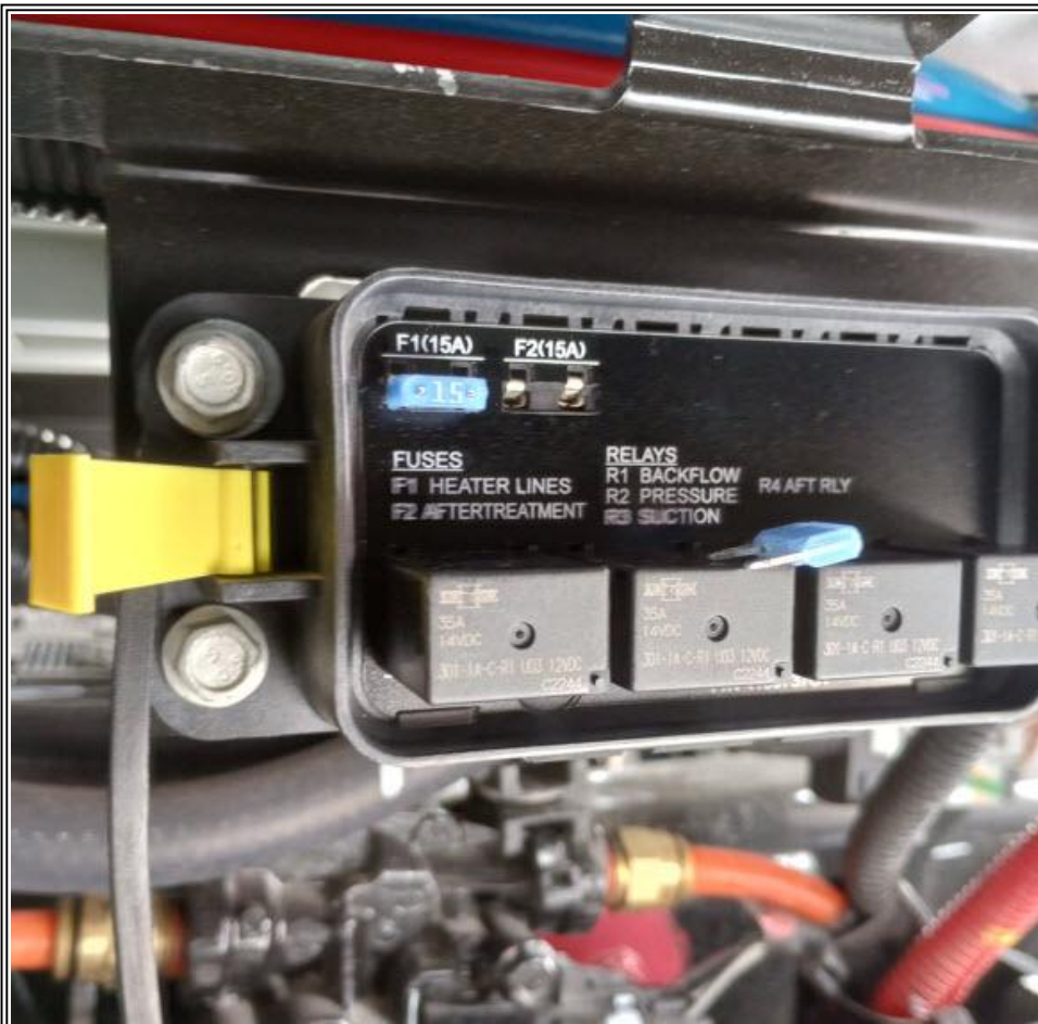
Figure 4: F2 Aftertreatment Fuse Loose in PDM Cover
