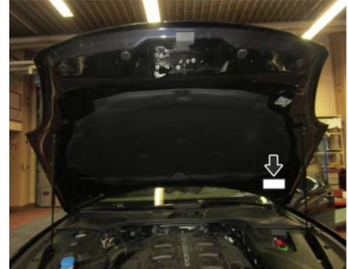
*Proof of Completion Label: specified position (Exemplary illustration — 718 (982) position accordingly)*
