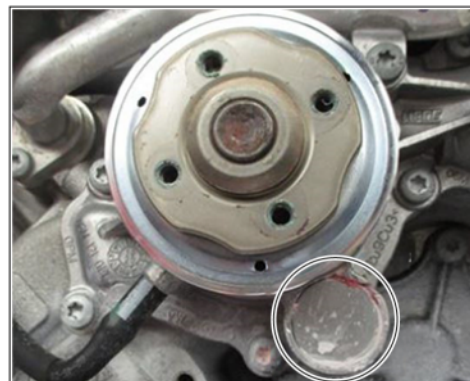
Traces of coolant on coolant pump
