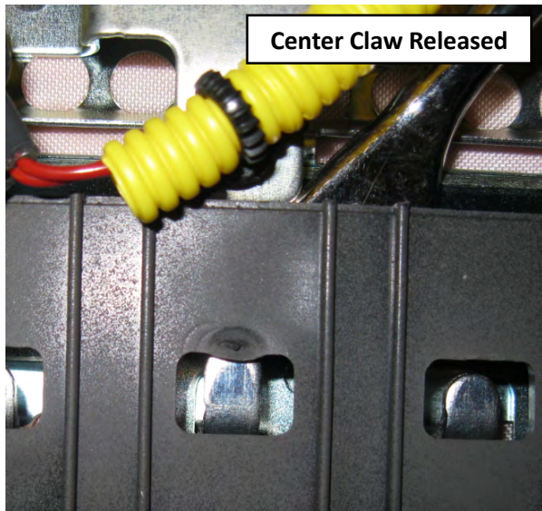
Trim Clip Removal Tool Inserted
