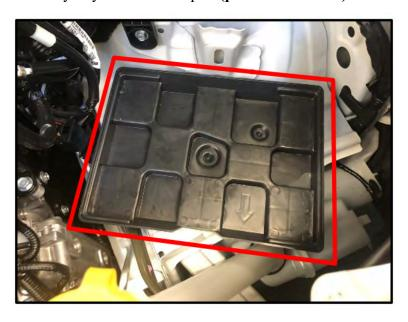
STEP 4: Install the NEW battery cover (p.n. 82123AN000) to the alternative replacement battery. Confirm the bottom of the cover is aligned flush with the bottom of the battery.
