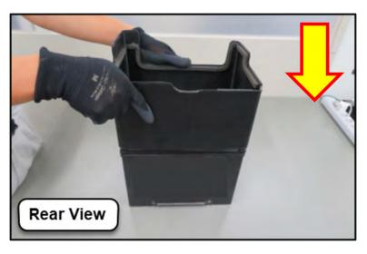
**STEP 5:** Install the replacement battery as per the applicable Service Manual: <u>Engine > STARTING/</u> <u>CHARGING SYSTEMS > Battery > Installation</u>
