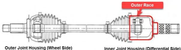
Inner Joint Housing (Differential Side)
