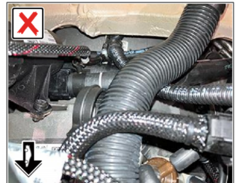
Previous position of control line for exhaust flaps
