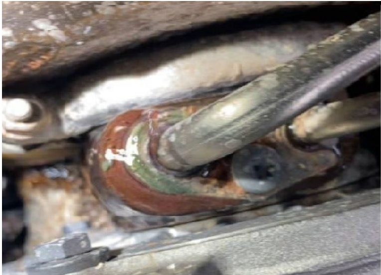
Figure 1: Coolant leak at the return lines to the turbocharger.
