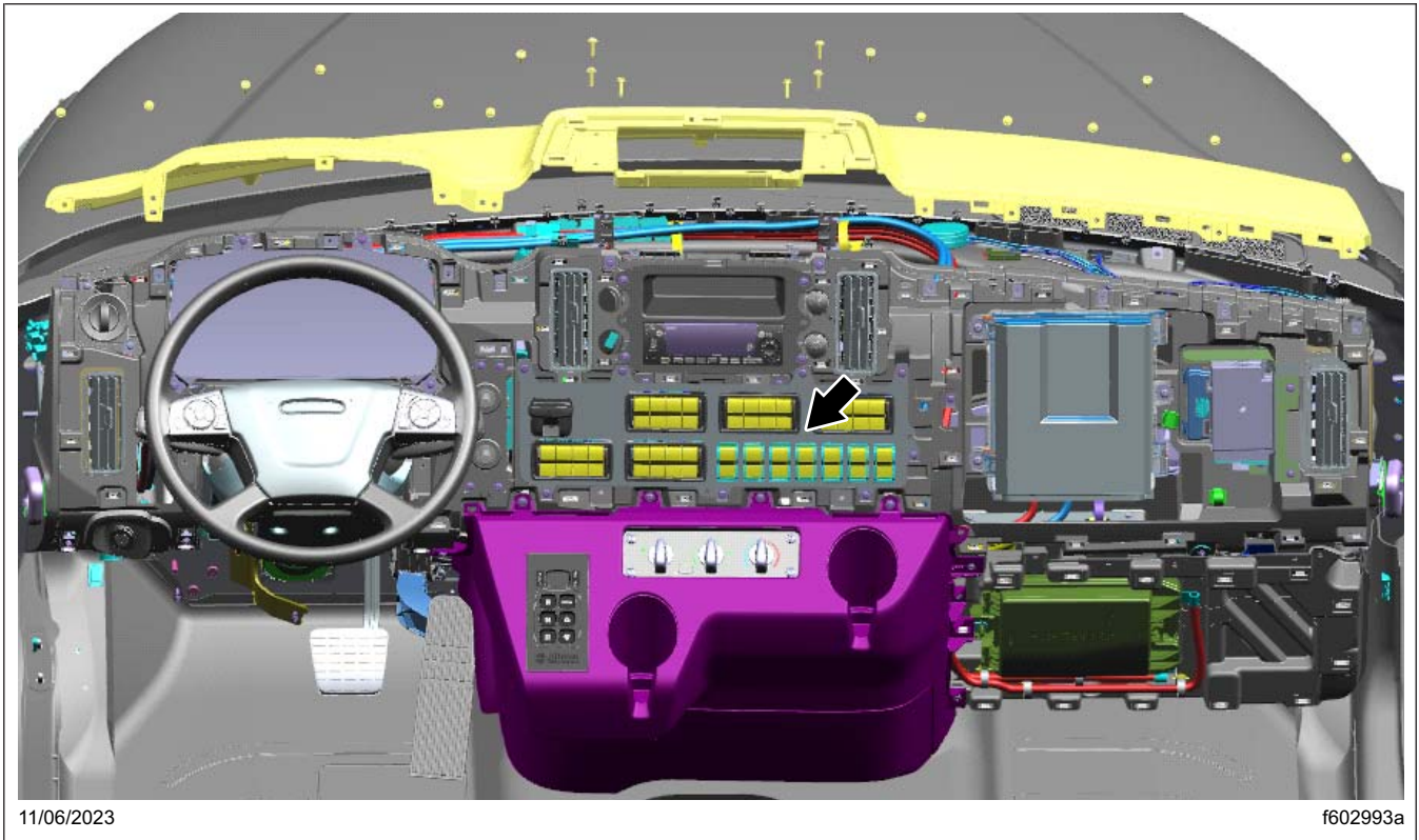
Fig. 11, Center Dash Switch Panel
