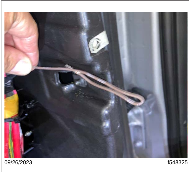
Fig. 35, Folding the Brown Wire
