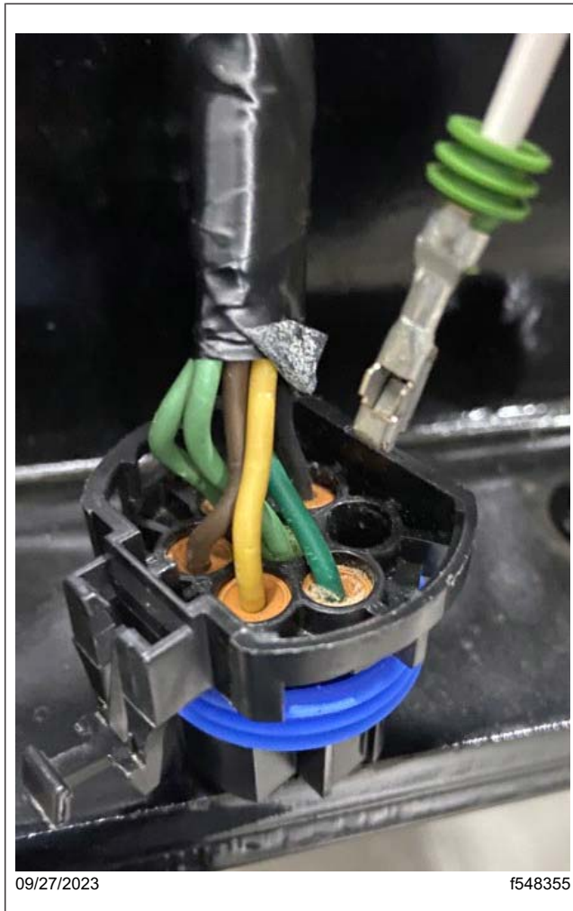
Fig. 71, Inserting the Wire into the Open Cavity of the Single Plow Light Connector
