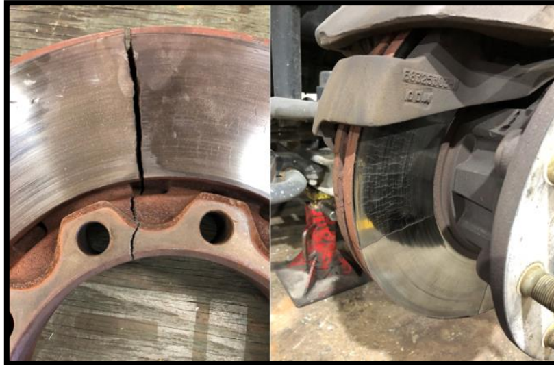
(Example of failed rotors)
