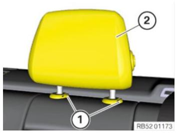
Install head restraint 2 into the guide sleeves, and depress the guide locks 1 to adjust height.
