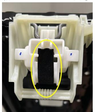
Apply felt tape 40 x 15 mm onto the plastic housing as shown.
