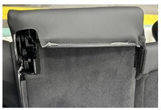
Install the 20% latch cover and trim retainer in the back of the upper 20% trim.
