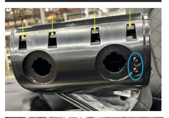
Carefully assemble the front head box cover by locking into the tabs shown with yellow arrows and the tabs on the side (*not shown in this view*).
