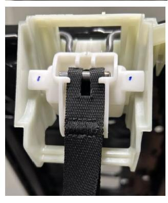
Install pull tab and its metal retaining pin into the plastic housing.
