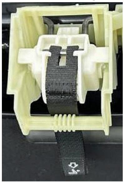
The metal pin that retains the pull tab may move within the plastic housing if manufacturing tolerances are too great.
