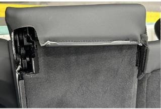
Remove the 20% latch cover and undo the trim retainer in the back of the upper 20% trim.
