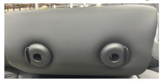
Follow Repair Instructions REP-52 26 394 to remove guide sleeve(s) for the head restraint.
