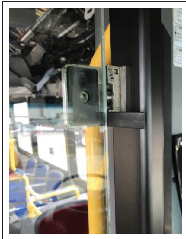
Figure 4 - Ensure 3mm Gap on Side mounts
