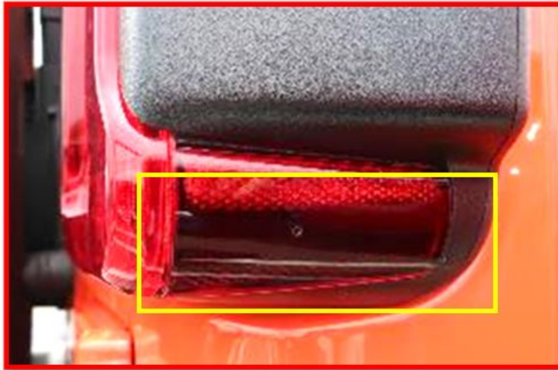
Fig. 2 Water Intrusion Side Marker
