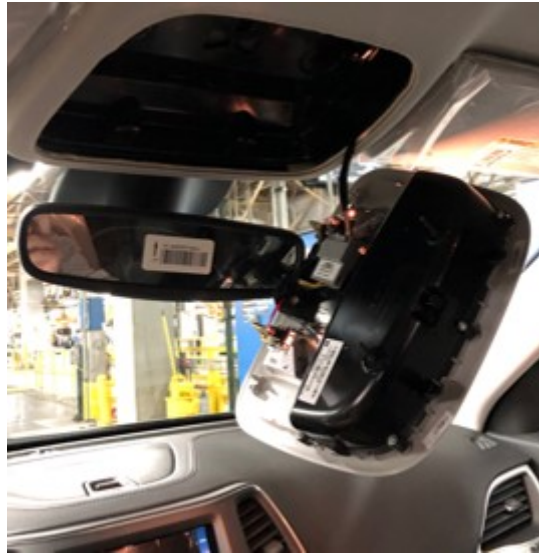
Fig. 1 Overhead Console Fall Out
