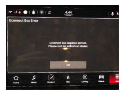
**Discussion**: To establish first time connectivity server connection, the TBM / radio needs to sync with vehicle manufacturing data and download a security certificate. Uconnect box requires service message will pop up if the certificate download failed.
