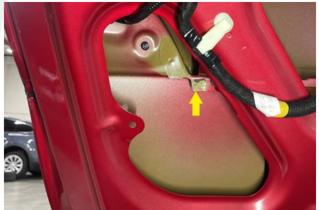
Figure 3 – LH factory foam removed from the liftgate assembly; RH similar
