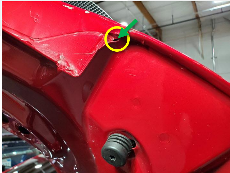
Figure 25 – Example of pin hole on the liftgate assembly
