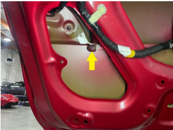
Figure 2 – LH factory foam inside liftgate assembly; RH similar
