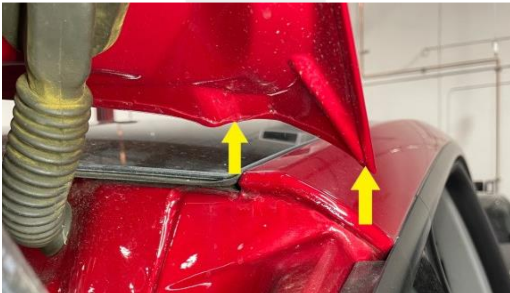
Figure 23 – Example of liftgate assembly seam
