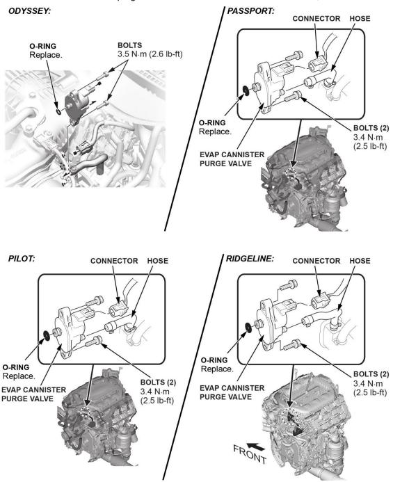
3. Replace with a new purge control solenoid, and then install parts in reverse order.
