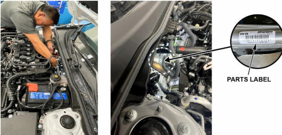
3. Inspect the label on the EPS gearbox and check the ID and part number on the label.
