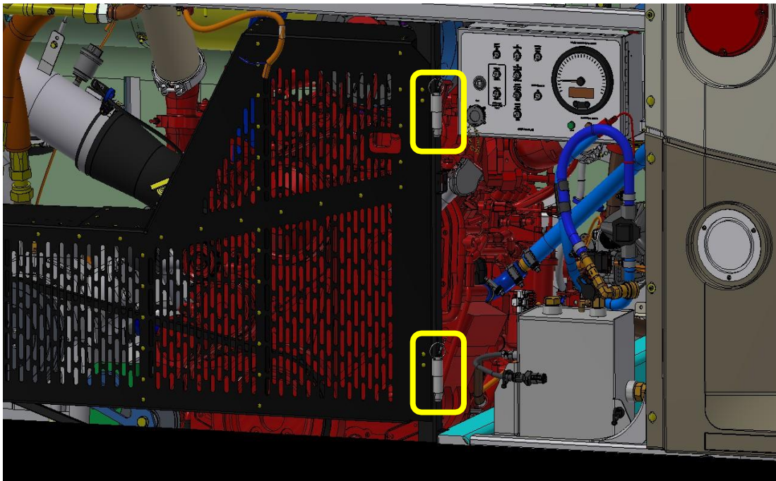
Figure 16 - Install Belt Guard and Adjust It
