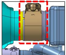
13. Ensure that the center muffler is mounted horizontally, then fully tighten the clamp.
