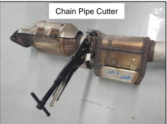
8. Remove any foreign substances, burrs, welding spatter, rust, and rough edges with a file or similar tool. Be sure to remove any debris that may have fallen into the catalyst.
