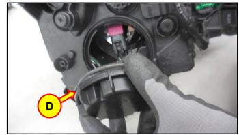
9. Shake the head lamp to remove the debris through the dust cover opening.
