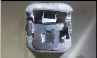
13. Insert the clip installation tool into the drilled hole.
