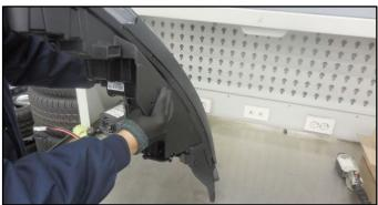
10. Insert a flat-head screwdriver into the hole to inspect the head lamp high beam function.
