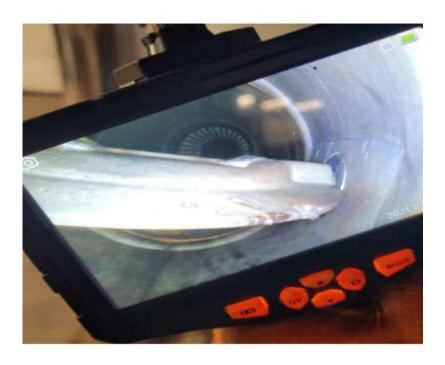
**4.2.** Check if the shaft rotates freely and make sure that the flap is not binding or sticking due to any debris, dirt, ice, or welding spatter, as shown in the pictures above.
