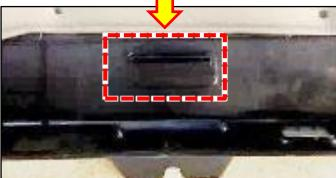
2. Measure 11 mm (7/16 inch) down from the top of the protrusion, and mark the area to be cut using a white marker.
