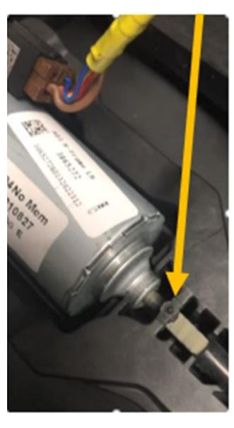
The electric motor for forward/back seat adjustment (SLV motor) may have become loose from its plastic mounting tray, allowing the drive cable mechanism to rub (arrow).
