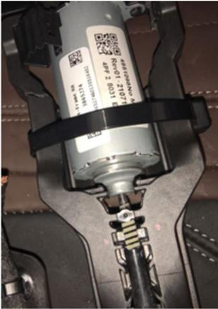
2, If it is not, secure the electric motor for the forward/back seat adjustment in place with a plastic zip tie.
