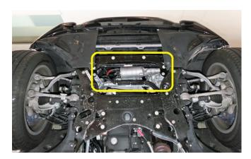
1. Raise vehicle on lift to access the steering gear (circled) beneath the vehicle.
