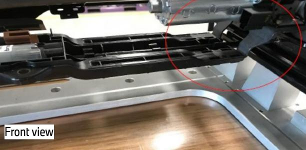
3. To make this repair the inboard flex cable and cover tube needs to be completely removed from the motor carrier tray and replaced. This will be shown in the next steps.
