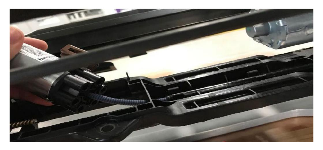
10. Move flex cable in the inboard direction so it is properly seated into the rail gearbox.
