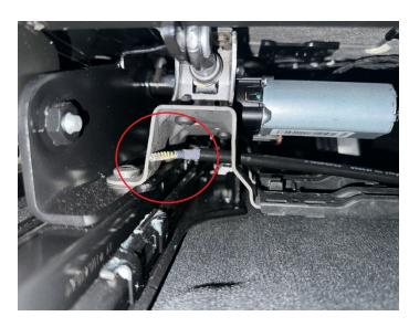
In vehicles equipped with the second row 60% / 40% split seat, the flex cable assembly can come out of the seat rail mechanism (circled). This stops the forwards and backwards travel of the seat.
