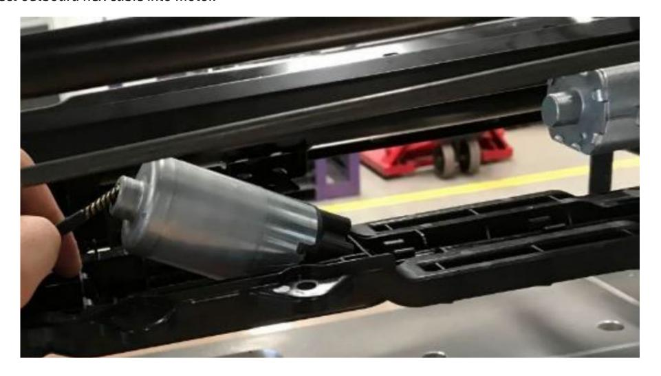
12. Once both flex cables are properly secured and aligned, use plastic cover piece to resecure motor. Make sure both spring clips are engaged.
