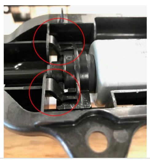
13. Test seat operation multiple times fully forwards and fully backwards on rails to ensure installation was correct and flex cables correctly engaged the rail gearboxes.
