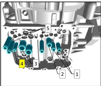
Install new bolts <arrows> from the repair kit and torque to 20 Nm + 90°.
