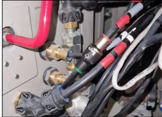
Figure 6: Orientation of single-check valve (green ring must be located at distribution block side)
