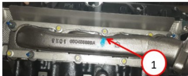
Fig. 1 Exhaust Manifold Crack Area
