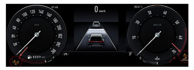
**Discussion**: At this time do not replace any parts or perform any calibrations for this concern. It is recommended to reassure the customer that this is normal behavior of the system to warn the driver of the temporary unavailability of the system. A software flash for the Forward Facing Camera (HALF Module) and the Instrument Panel Cluster (IPC) is expected to be released in Quarter 1 of 2024.
