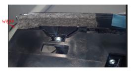
Add Two Pieces of Felt Tape to the Cupholder 10mm x 70mm x (0.5 to 1.0 thick)
