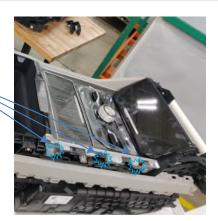
Disconnect shifter wiring.
