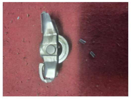
Note: Inspect the cylinder head area for any loose roller bearings and remove before reassembly. Each of the roller followers will have a total of 10 roller bearings.
