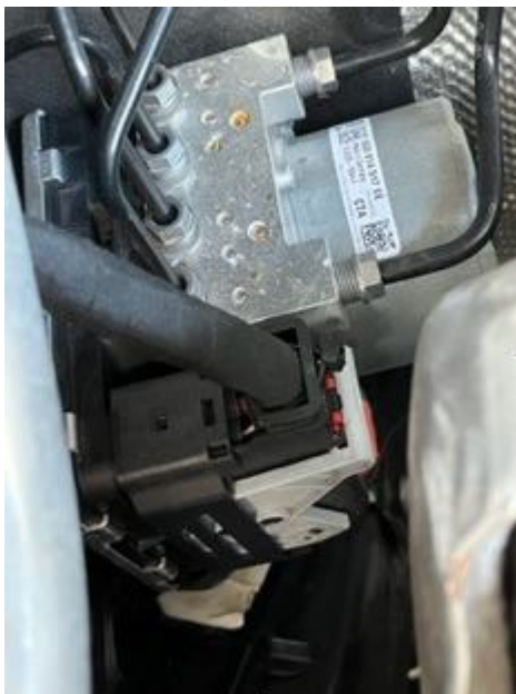
Figure 1: ABS hydraulic unit / ABS control unit connector.
