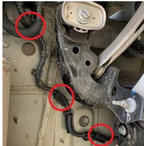
Figure 2: Sleeves installed on the activated charcoal filter line.
