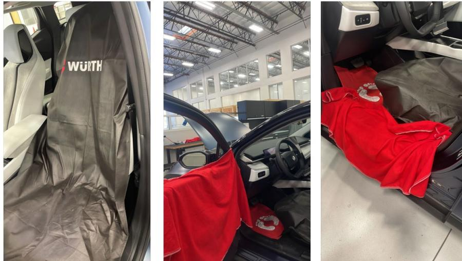
Figure 1. Example of interior trim cover protections
