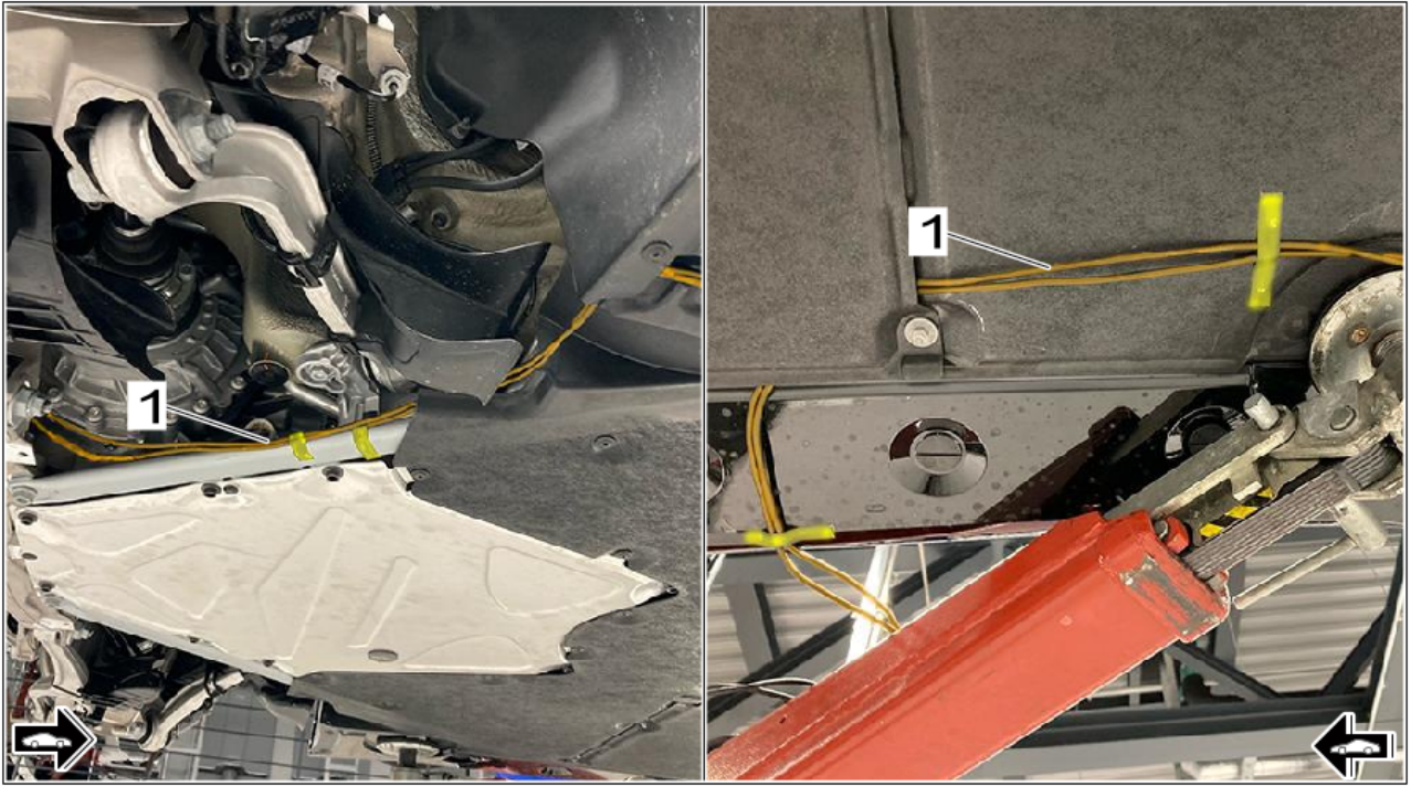
Example of routing / fastening underbody
