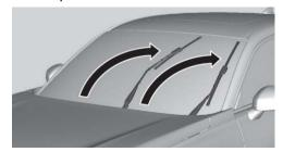
In this position you can better access the wiper blades for replacement or to lift the arms away from the windshield to prevent blockage by snow and ice buildup.
