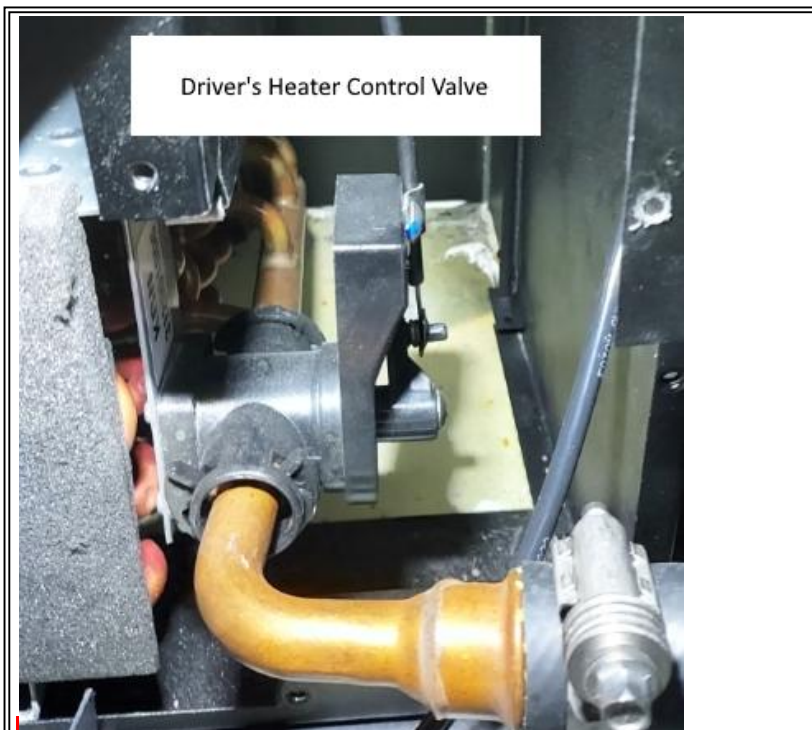
Figure 4: Heater Control Valve Location
