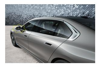
While driving at highway speeds, wind noise can be heard from the exterior mirror assembly. In some cases, this can be also felt in the B-pillar area.
