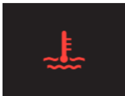
Figure 1: Warning lamp for low coolant level.
