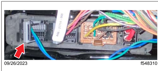
Fig. 40, XMC2 X1 Connector Latched
