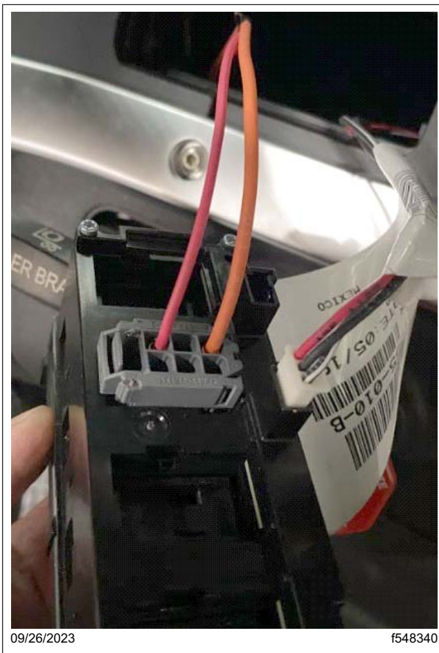
Fig. 62, Connector Plugged into the Back of the Plow Light Switch
