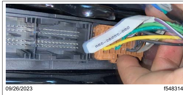
Fig. 44, XMC2 X3 Connector Removal
