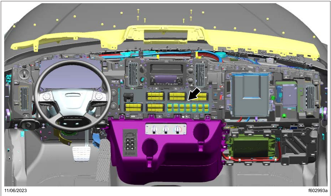
Fig. 11, Center Dash Switch Panel
