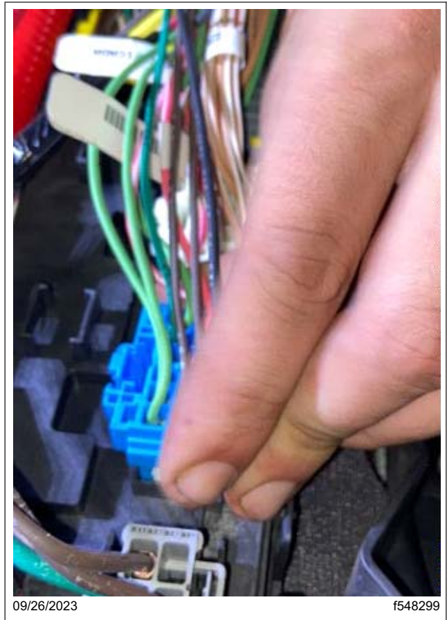
Fig. 31, X2 Connector Plugged into the SSAM
