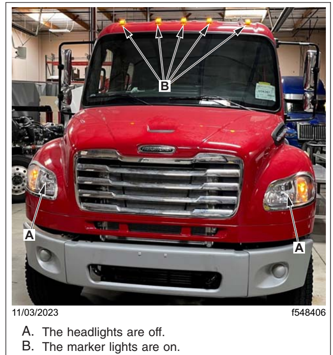
Fig. 90, Verifying the Headlights Turn Off and All Other Marker Lights Remain On After Turning On the Plow Light Switch
