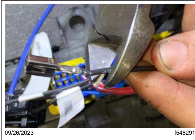
Fig. 23, Cutting Off the Terminal
