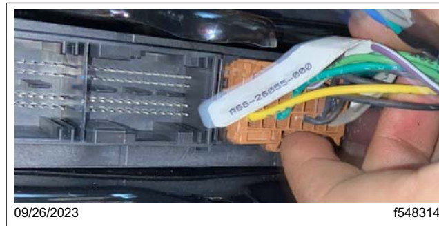
Fig. 46, XMC2 X3 Connector Removal
