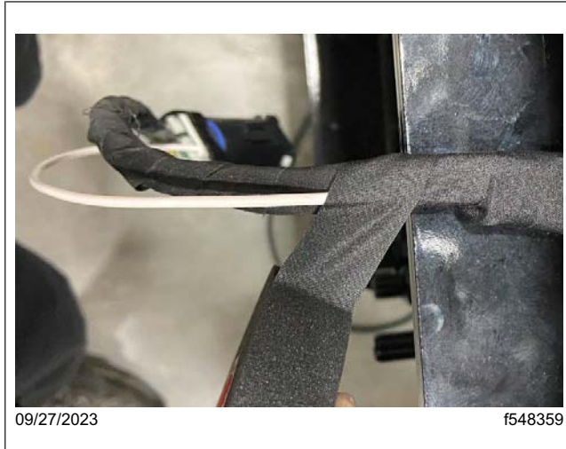
Fig. 91, Wrapping the Exposed Wiring with Fabric Tape
