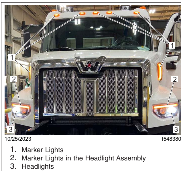
Fig. 127, Verifying that the Headlights and the Markers Turn on Prior to Turning on the Plow Light Switch
