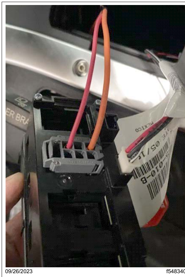
Fig. 72, Connector Plugged into the Back of the Plow Light Switch
