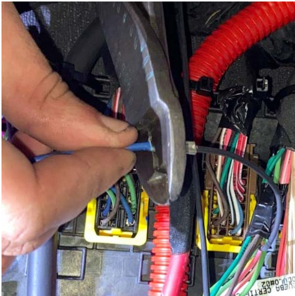
Fig. 33, Splicing the Wire
