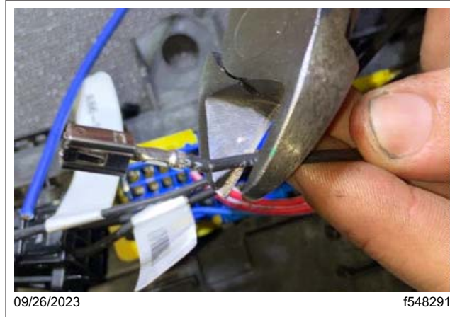
Fig. 23, Cutting off the Terminal
