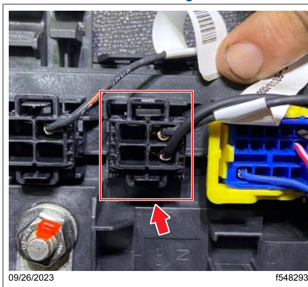
Fig. 25, X10 Connector Plugged into the SSAM
