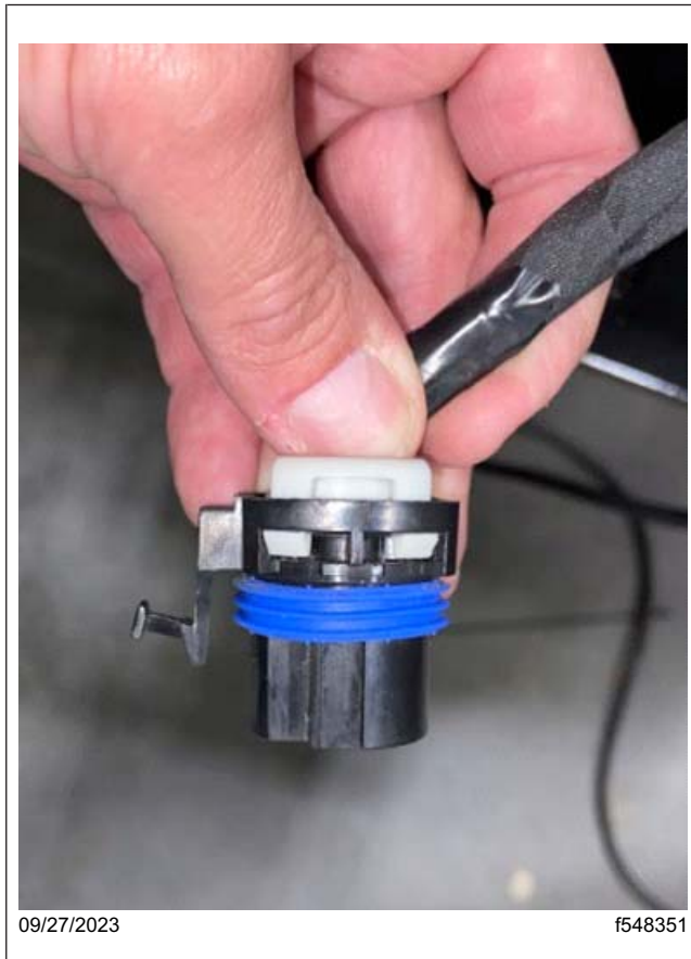
Fig. 83, Single Plow Light Interface Connector with the Cover Removed
