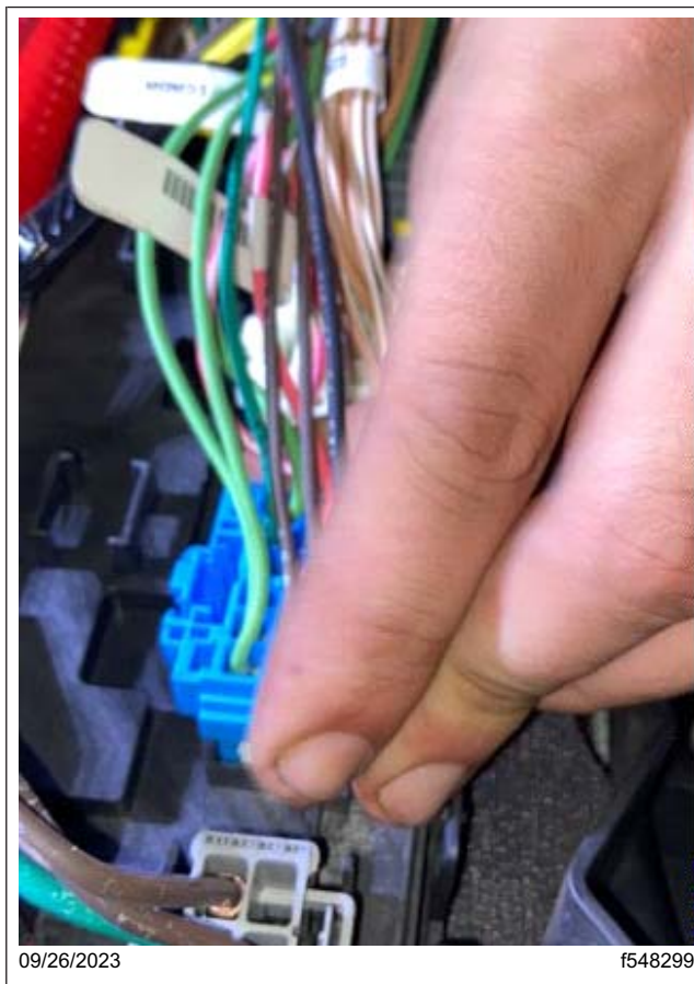
Fig. 31, X2 Connector Plugged into the SSAM
