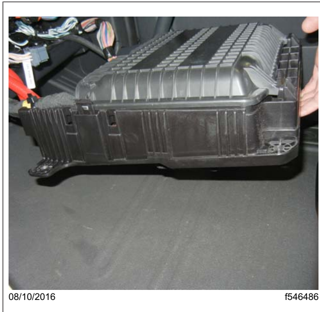
Fig. 12, VPDM Lowered to the Floor
