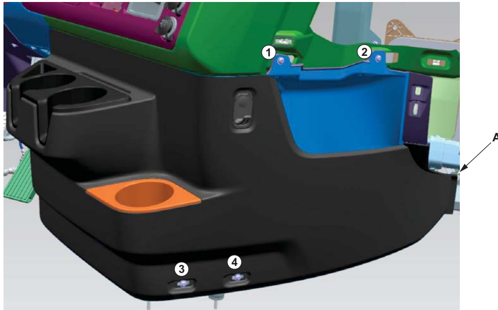
Fig. 11, Center Dash Cover Removal
