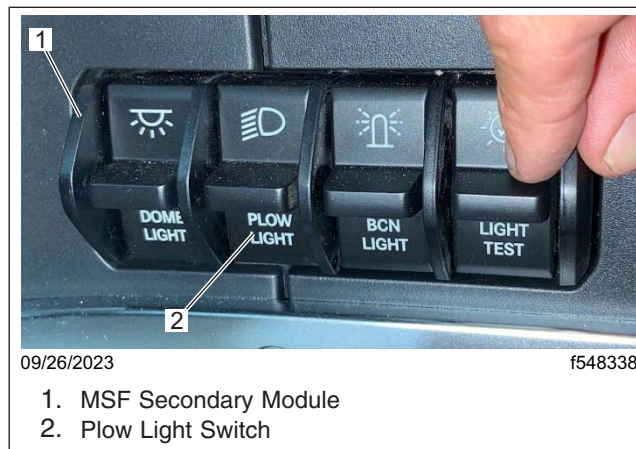
Fig. 70, Plow Light Switch in MSF Secondary Module
