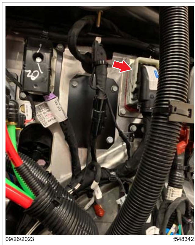
Fig. 74, 104-Way Bulkhead Connector Location
