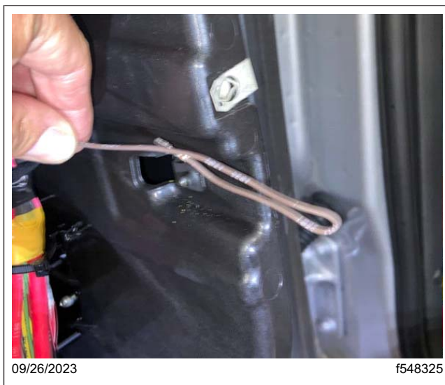
Fig. 57, Folding the Brown Wire
