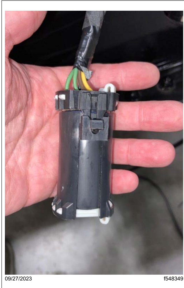
Fig. 81, Single Connector Plow Light Interface
