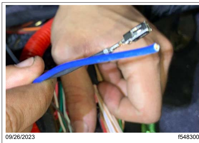
Fig. 32, Wire Removed from Cavity 6 of the SSAM X2 Connector and the Shorter Blue Wire, to be Spliced Together
