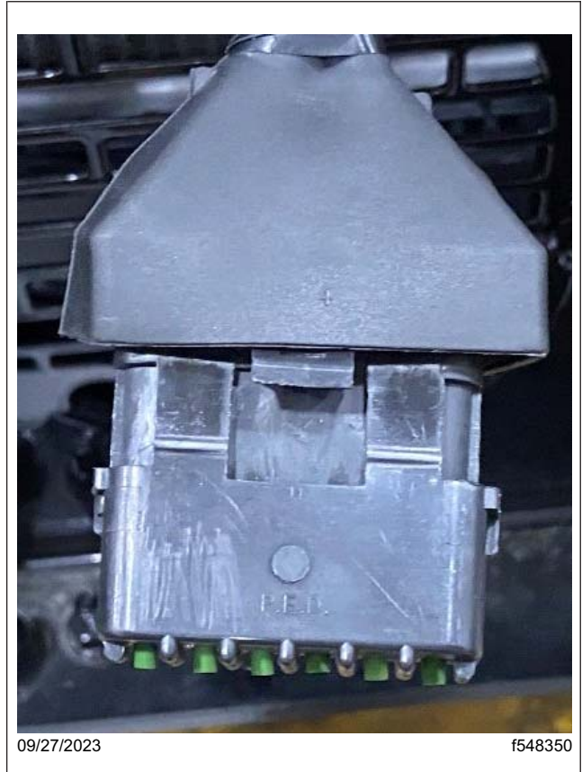
Fig. 82, Dual Connector Plow Light Interface (one connector shown)
