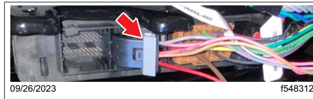
Fig. 44, XMC2 X1 Connector Latched
