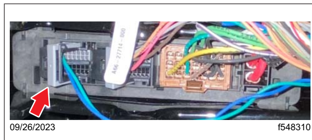
Fig. 42, XMC2 X1 Connector Latched
