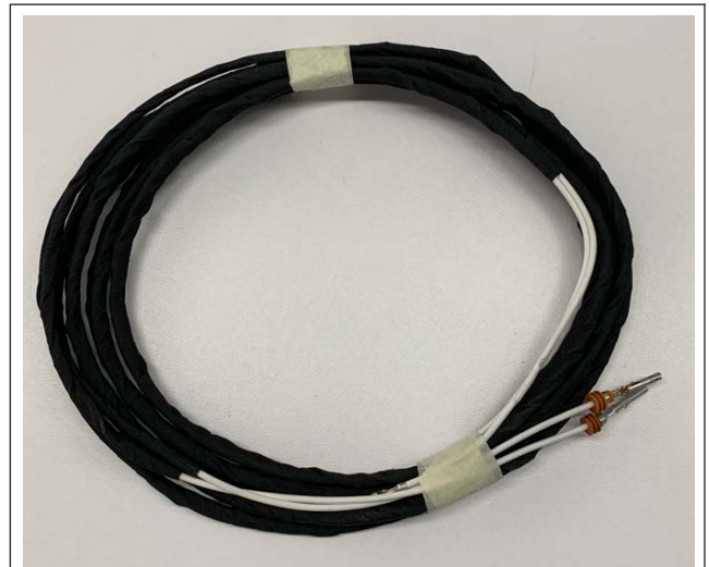
Fig. 2, Underhood Plow Harness (TSU CT44FRT034)
