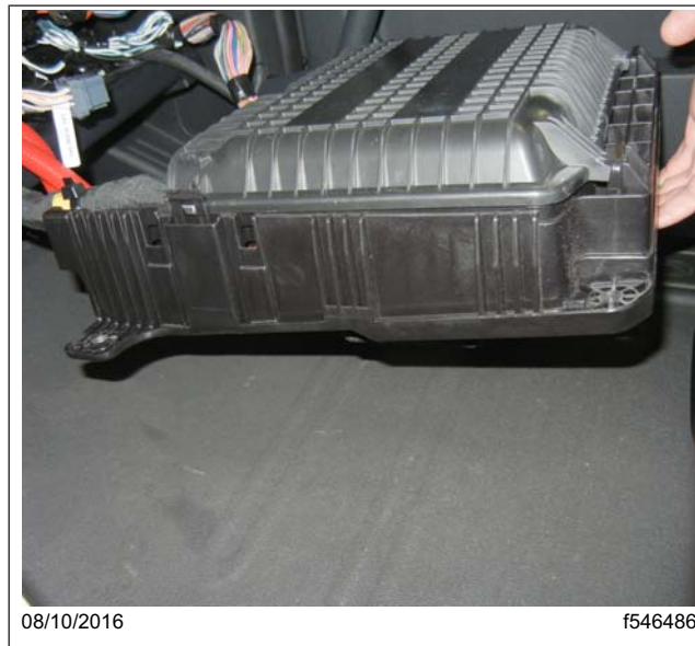
Fig. 11, Lowering the VPDM to the Cab Floor
