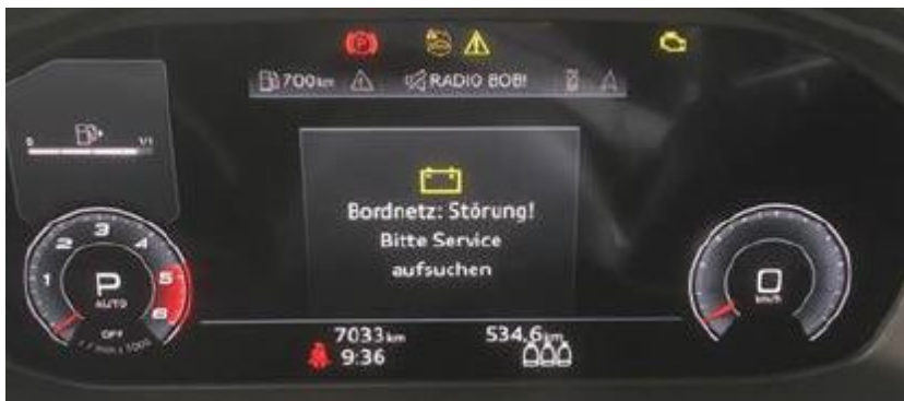
Figure 1. Yellow electrical system warning lamp.
